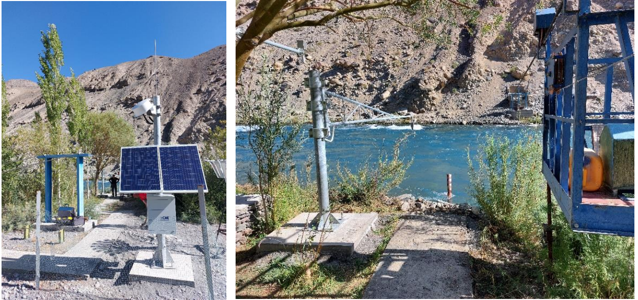
A water level gauge downstream of the dam
